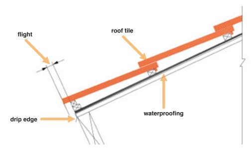
The distance from the eave batten (the first) to the second one will depend on the flight you want to give the roof over the eave line, which is normally between 4/5" and 2".
